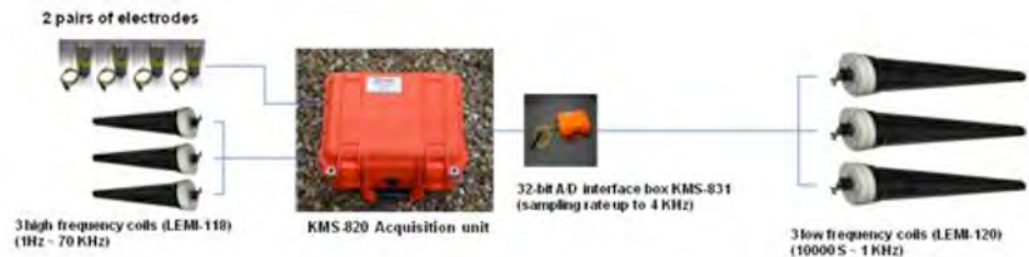
Figure 1: Application example of KMS-831 for simultaneous sampling for low and high signal band in MT survey
